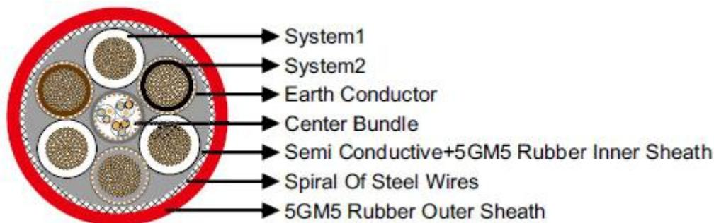
**System1 (1.8/3kV or 3.6/6kV):** Flexible stranded tinned copper conductor with heatresistant3GI3 rubber based on EPR, easy strippable outer conductive layer.
